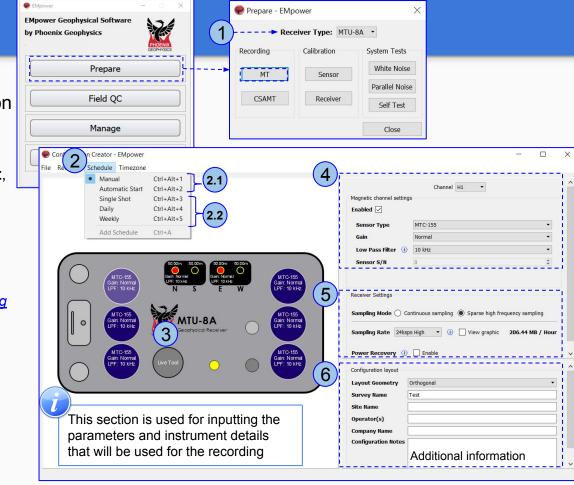
To use the magnetic sensor data from a different recording or use a remote reference, all recordings **must** have a matching Sampling Mode and Sampling Rates. Otherwise, EMpower will not allow to process the data using borrowed channels or remote reference
